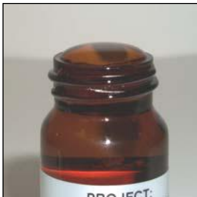
Figure 7. Example of Bottle Where Reverse Meniscus is formed
